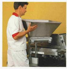
The hopper can be quickly removed for cleaning. For use with mixes such as fondant or chocolate, an easily removable heated hopper jacket can be supplied.
