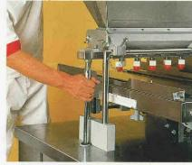
The drive is quickly engaged through this telescopic fitting when a rotary template is selected for use.
